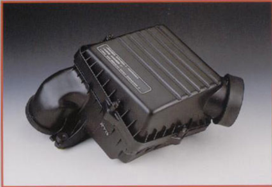
CIVIC 92-95 空氣濾心蓋總成 EG8/K600 CASE ASSY., AIR CLEANER SK2552-CV92 17201-PO7-000
