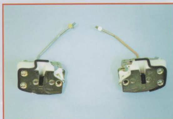
CIVIC 96 3 DOOR 車門六角鎖 SK6141-CV96 3D 72110-S00-A01 (FR) SK6142-CV96 3D 72150-S00-A01 (FL)
